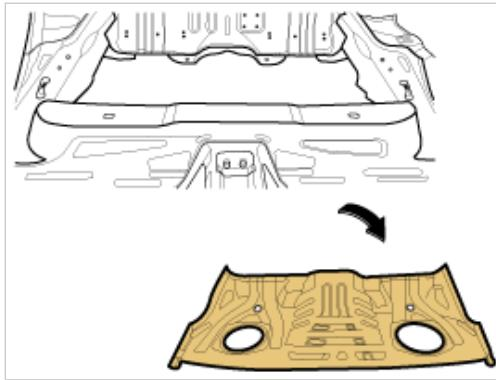
4. To remove the rear floor side member assembly, drill out all welding points of the rear floor center cross upper member.
