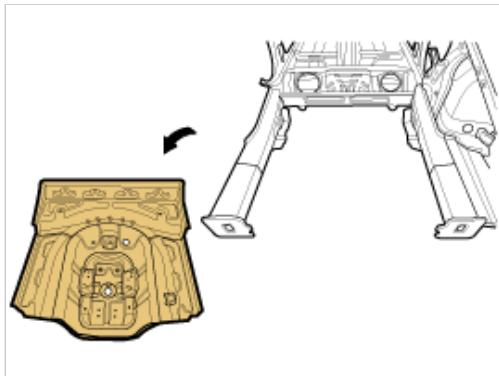
2. To remove the rear floor side member assembly, drill out all welding points of the rear floor panel.
