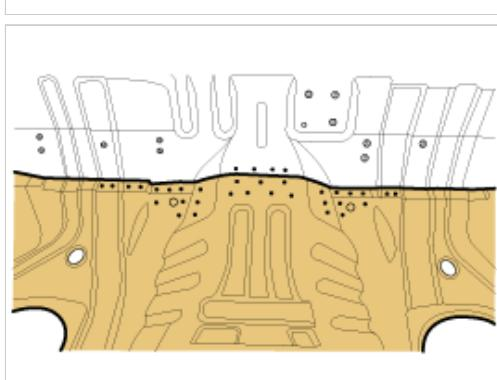
21. Install the rear floor panel.(Refer to the rear floor panel repair procedures)
