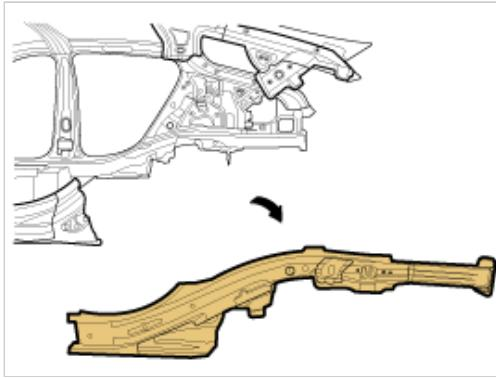
10. After removal, remove broken panel parts from welding area.
