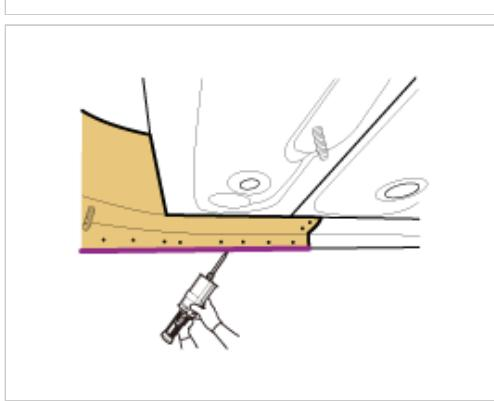
6. Cut and process new panel before installing on body.
