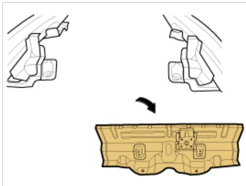
8. Drill out all welding points of the rear floor side member assembly.
