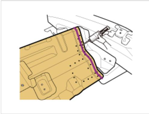
11. Cut and process new panel before installing on body.
