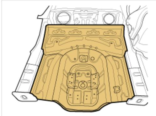
22. For plug welding, remove welding bead with a grinder and clean the welding area.
